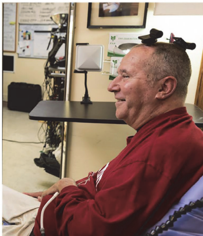
A participant in the BrainGate clinical trial uses wireless transmitters that replace the cables normally used to transmit signals from sensors inside the brain. Credit: Braingate.org
